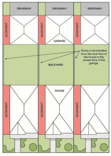
Note: Sheds and other structures are NOT permitted within the easement. Fences should be installed so that the bottom rail sits at least 1" above the ground to allow for proper drainage.
